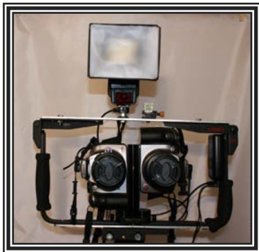
My Stereo 3- D Rig Note the 2 cameras. Flash and Microprocessor Controller (on the right side)
